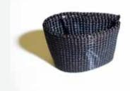
Taking a 2 3/4 inch piece of 1'" Type IV create a 1' loop and mark at 5/8' from outside edge.
