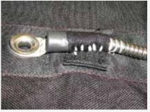
Make three more turns around housing and tie off to hold in place. Cut excess hand tack thread.
