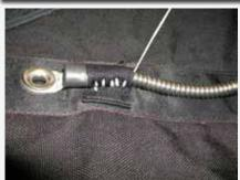
Hand tack terminal end of housing. Make five turns of hand tack around housing in direction of housing channel.
