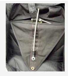
Place new housing with terminal end through drogue loop, positioning the terminal end of housing over original grommet hole.
